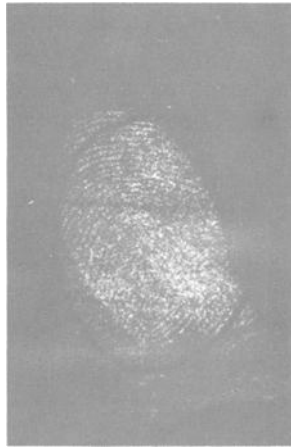
FIG. 2—Latent fingerprint on strongly fluorescent (yellow) paper dusted with Sirchie DP 002 powder and detected by laser in the phosphorescence mode of Fig. 1.
